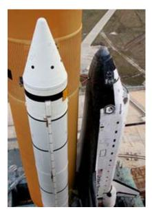
In addition to the solid rocket motor, the booster contains the structural, thrust vector control, separation, recovery, and electrical and instrumentation subsystems.
